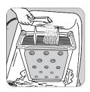
4. Clean the rubber seal round the condenser cabinet and in the inner part of the small door with a damp cloth.
